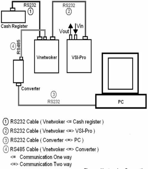
**Figure: Vnetworker Connection Diagram**
